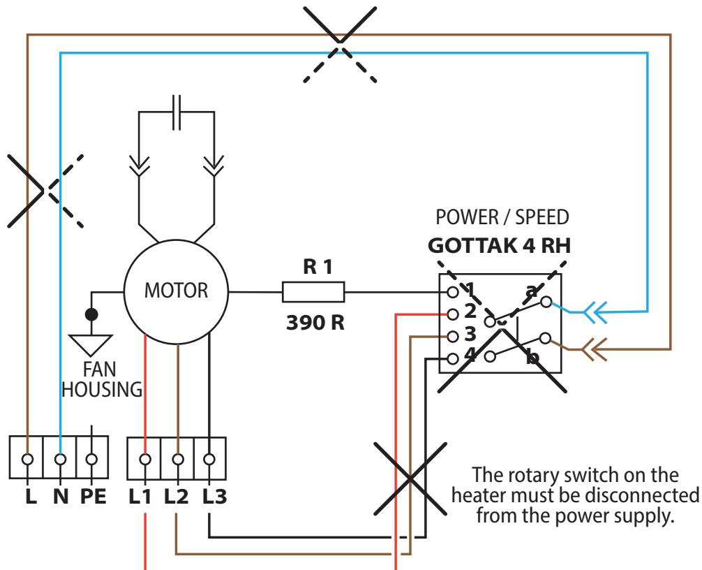
**Wiring diagram** for controlling the Saunum Primary or Premium series heater with Sauna LEIL control unit
