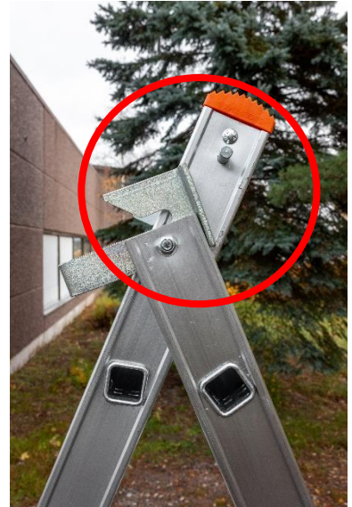
Hinge pin incorrectly placed Do not climb onto the ladder!
