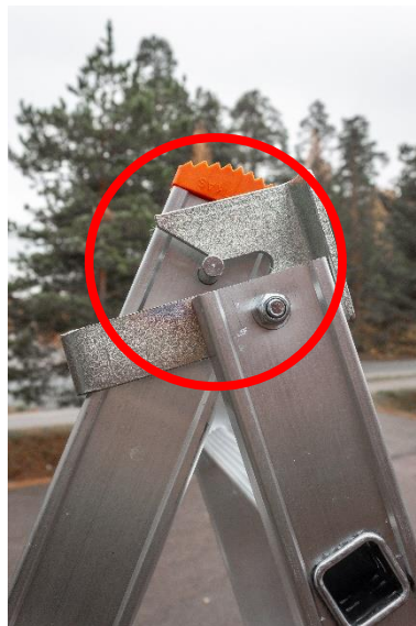
Hinge pin incorrectly placed Do not climb onto the ladder!
