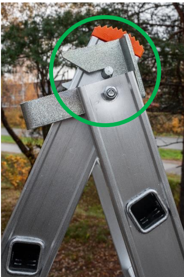
Hinge pin correctly in its slot It is safe to use the ladder!
