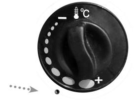
Determine the reason for the stove's overheating. The cause may be due to too densely placed sauna stones, the position of the stove, or incorrect ventilation. The stones should prevent a direct view of the glowing-red heating elements to the sensor. If the stove overheats, rectify the problem before using the stove again. The reset button is located below the thermostat switch.
