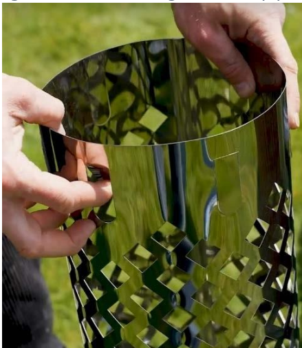
Figure 17: Sheet metal springs for the heat shield
